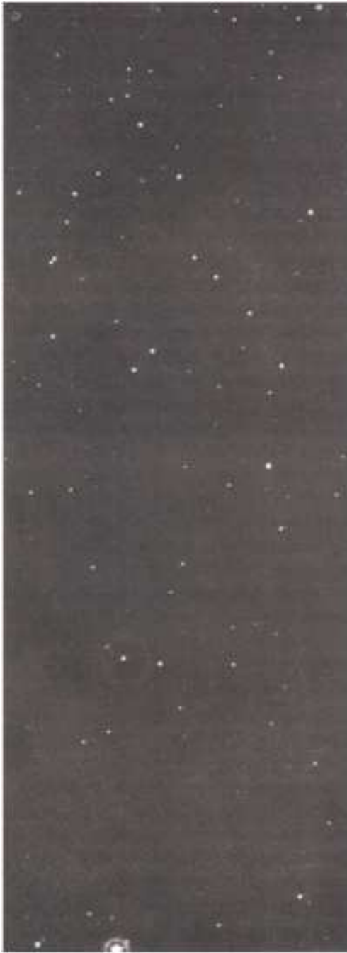
Fig. 9. The plate No. 2996, October 10, 1953, shows the region of the sky north to the star 56 Cygni, which is visible at the lower margin and whose regular figure of the diffraction image can be appreciated. Star images are circular and completely coma free up to the edges of the field. 1 arcmin = 3 mm at the scale of the original 9x24cm plate.
